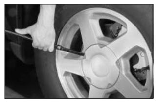
Position the chisel end of your wheel wrench in the notch of the center cap and pry off the center cap.
